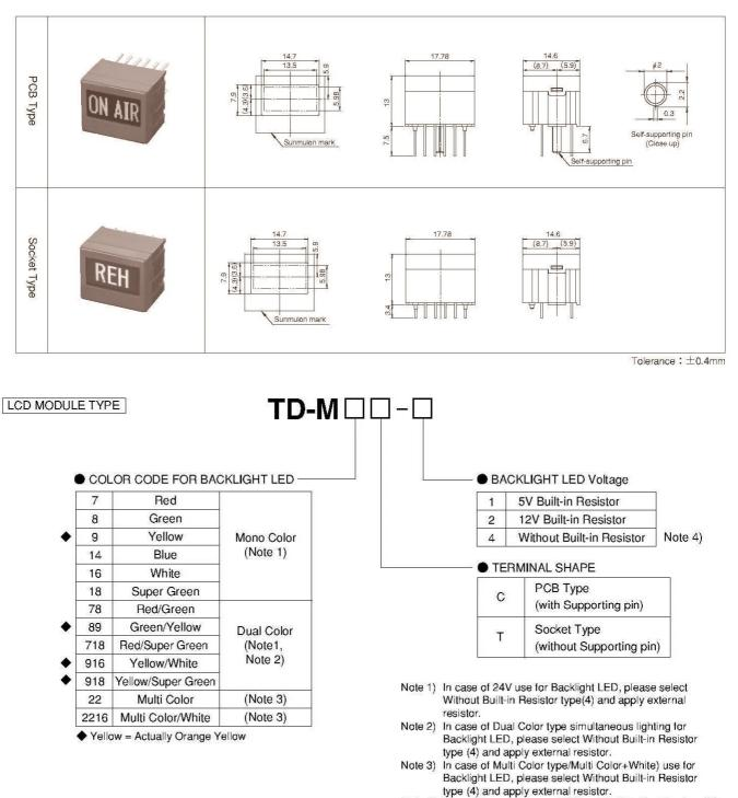
Note 4) Connecting arrangement Without Built-in Resistor type (4) is all the same.
